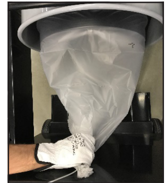
10- Pull the bag and place at the edge the band to create a new one. If necessary use two bands.
