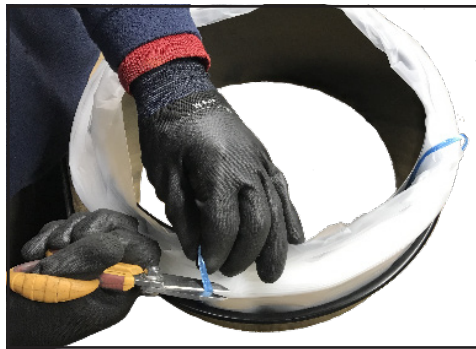
5- Cut and remove the Infinity Bag closing bands.
