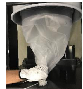
9- Pull the bag and place at the edge the band to create a new one. If necessary use two bands.
