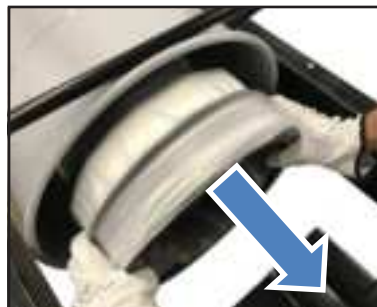
3- Remove the Infinity Bag container and any waste.
