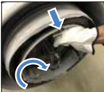
2- Pull and rotate the retaining pins of the Infinity bag container in order to unfasten them.
