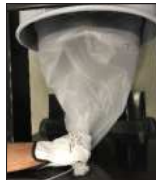
10- Pull the bag and place at the edge the band to create a new one. If necessary use two bands.
